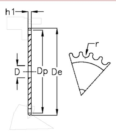
C = 2 D = 30 De = 700.6 Dp = 691.36 For chain size = 3/4 x 7/16 For chain type = 12 B-1 h1 = 11.1 Sumber of teeth = 114
